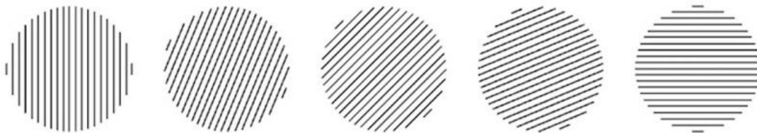
Figure 2.10 Illustration by author of each state of day/rotation angle ( 22.5^\circ ) of polarizing film.
