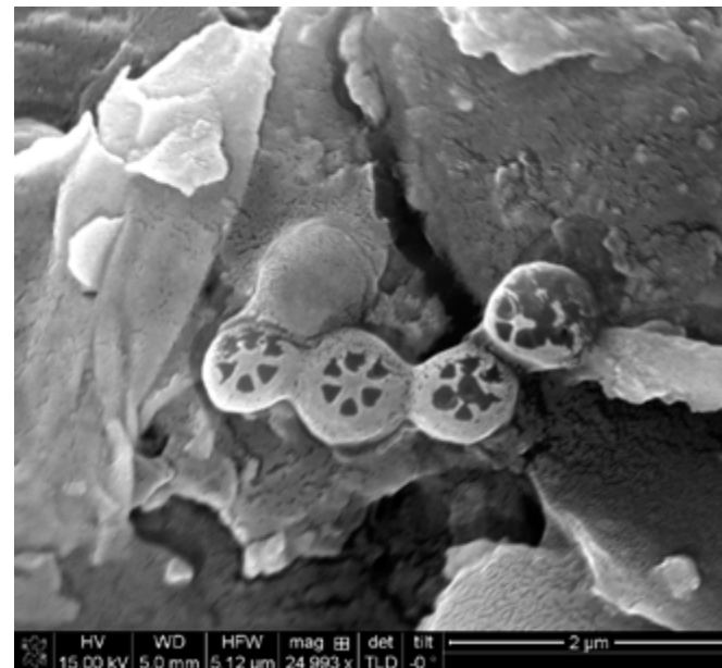
All four bacteria are marked with this triangular pattern testing different time intervals which determine the quality of the pattern. The two bacteria to the left had the best time intervals.
