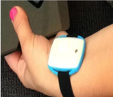
**Fig. 3:** A vibrator in the plastic holder mounted on the left wrist.
